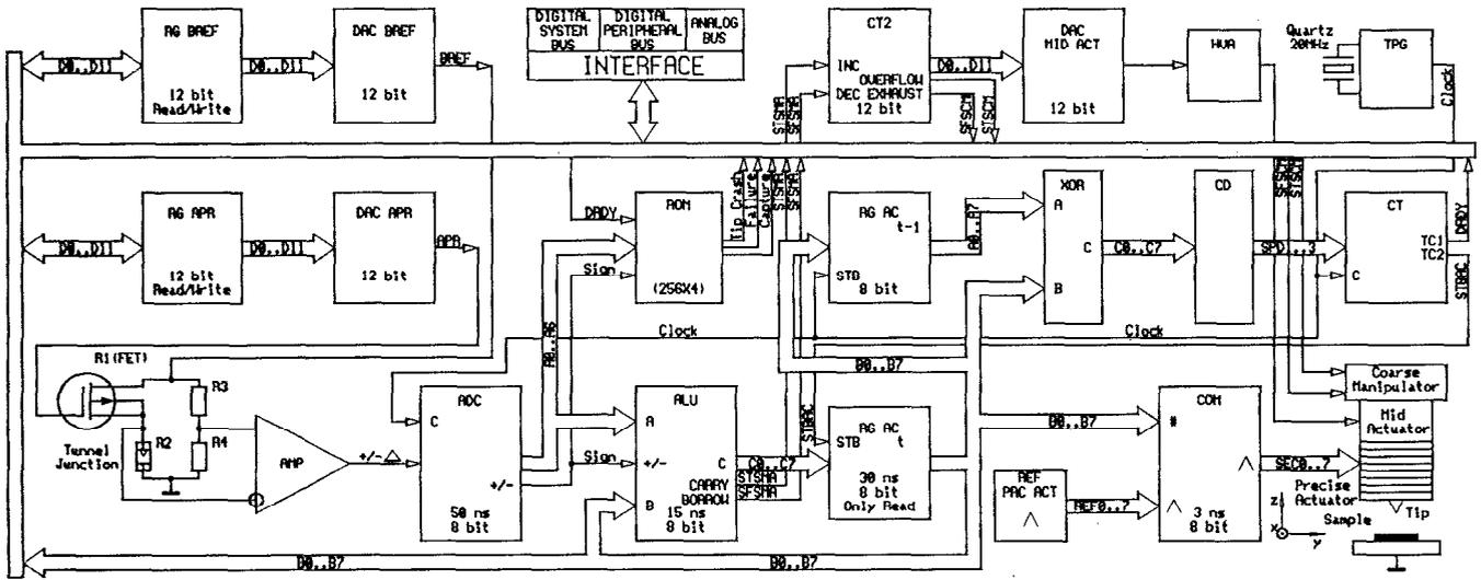
FIG. 3. Feedback loop functional flow chart.
