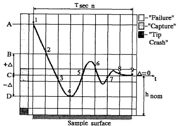
FIG. 5. Formation of the  $\pm\Delta$  displacement. Ranges of states "Tip Crash," "Failure," and "Capture." Transitional process of the actuator.
